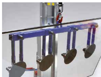
Manual gas suction unit for upright glazing
