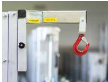
Load hook / adapter with swivel hook for gas suction unit
