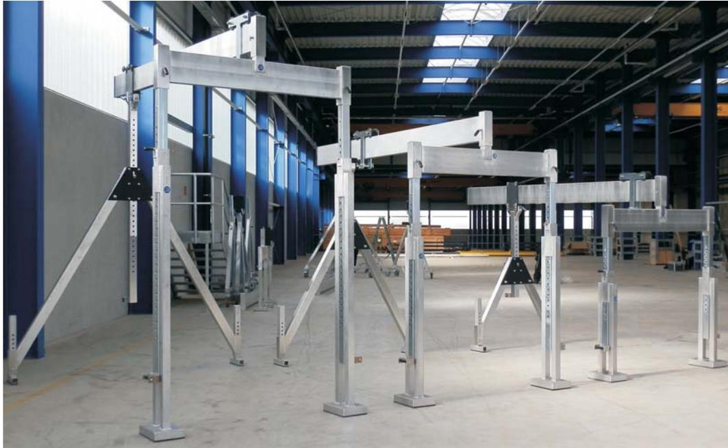
The lateral stand comes into use when the standard stand can't be positioned directly behind the load
